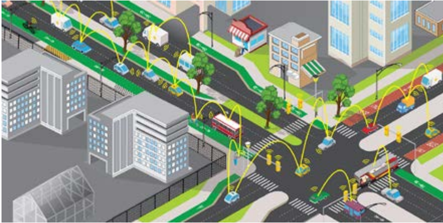
Figure 1 - Networked driving: vehicles communicating directly with each other and their surroundings to operate more safely - Image Source: WSP
