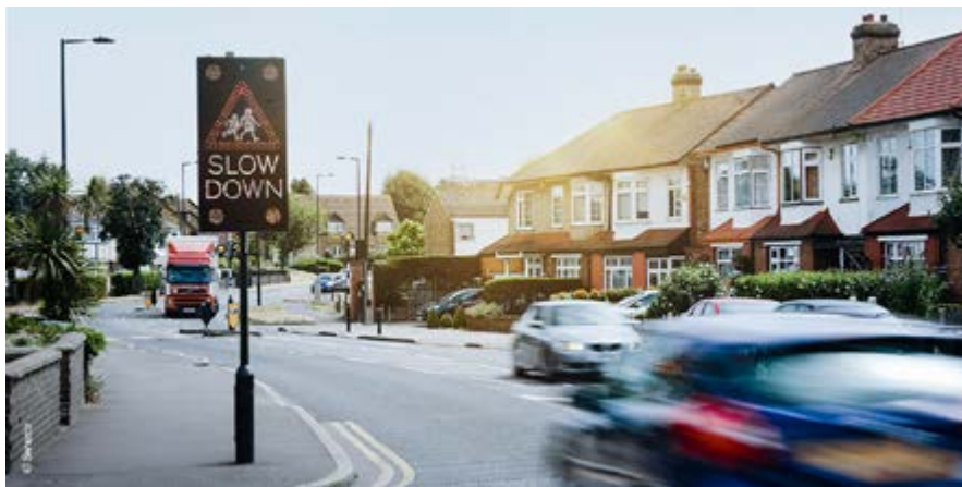
Figure 6 – Vehicle-activated sign to encourage compliance with speed limits (photo: courtesy of Swarco)
