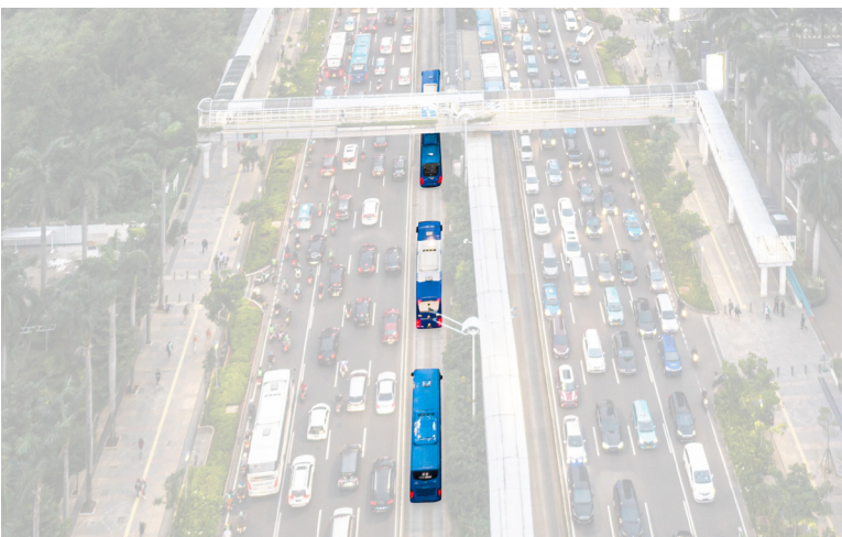
Figure 14: A bus platoon in Jakarta, one of the largest BRT systems in the world. Dedicated BRT laneways provide an ideal ODD for bus platooning with the opportunity to significantly increase capacity at a potentially lower cost than LRT can provide
