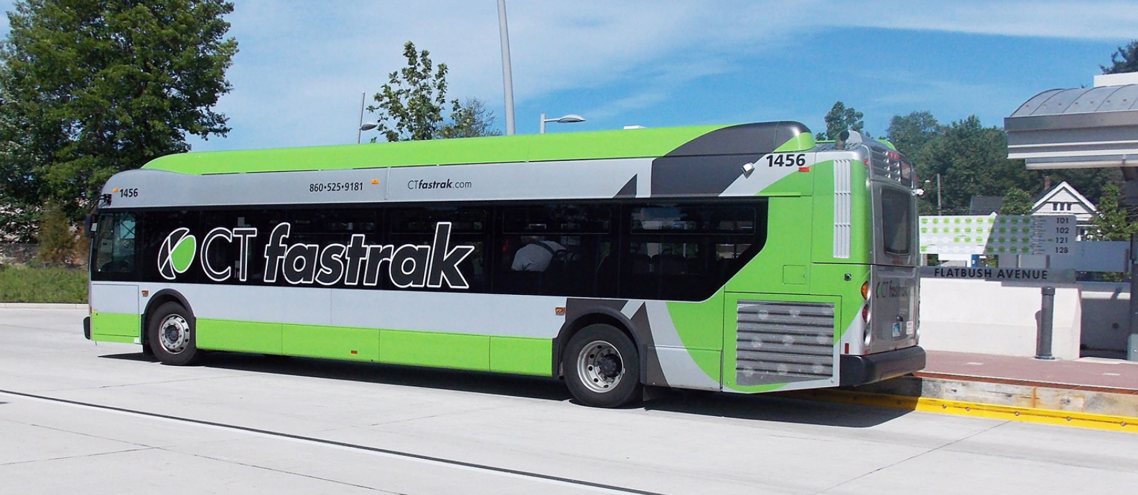
Figure 17: CTfastrak BRT System will test bus platooning and precision docking beginning in 2022 with three New Flyer Xcelisior AV™ buses. Image courtesy of New Flyer
