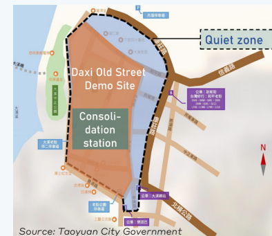
A conceptual plan of the Daxi Eco-logistics Demonstration project. 277 It includes a micro-logistics hub and quiet zones with lower speeds and traffic management.
