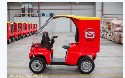
NZ Post has 450 Paxters in its fleet. 237 These small vehicles carry loads of up to 200kg but are still small enough to be used on the footpath and can easily navigate the hills of Auckland. 238
