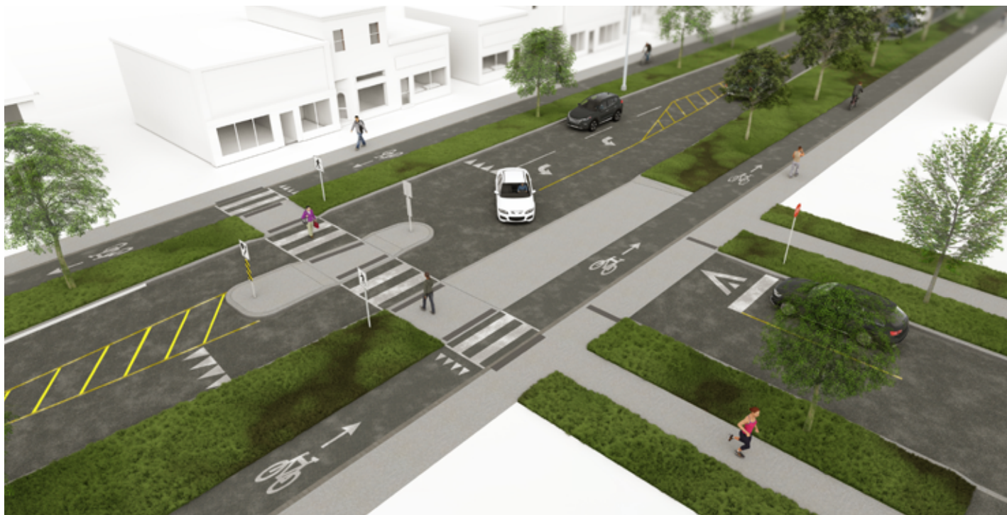
Figure 7: Rendering of a continuous sidewalk at a T-intersection (Hamilton Complete Streets Design Manual).
