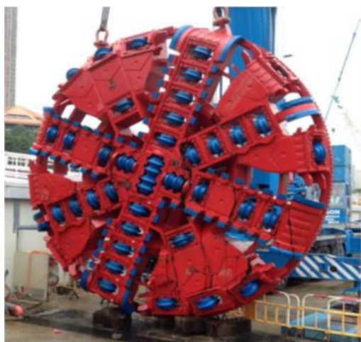
Figure 7. The cutterhead, equipped with discs, scrapers and bucket lips
