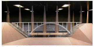
Figure 3 - Full aeroelastic model of the bridge in a wind tunnel
