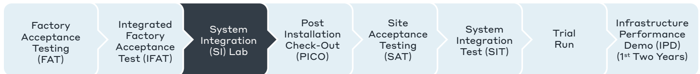
Figure 2 – Systems integration process with the systems integration lab at the core (before field installation) for cost savings and schedule compliance. The SI lab enables the integrated verification of products and configuration before deployment, to prevent regressions and delays.
