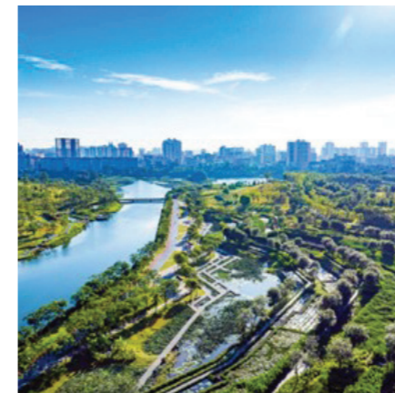
Figure 8. Meisha River Corridor, Haikou City, 2016. Terraced wetlands are densely covered with various plants that remove nutrients from primary treated wastewater. 147
