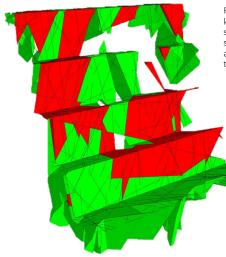
Figure 1: DFN based kinematic wedge stability analysis showing stable (green) and unstable (red) true blocks
